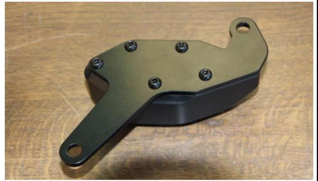
Insert the supplied spacer sleeves into the frame. Secure the crash pad to the frame with the washers and screws supplied.
