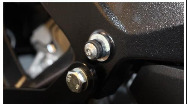
Attach the spacer roller to the frame with the supplied screw. **Right and left sides are identical.**
