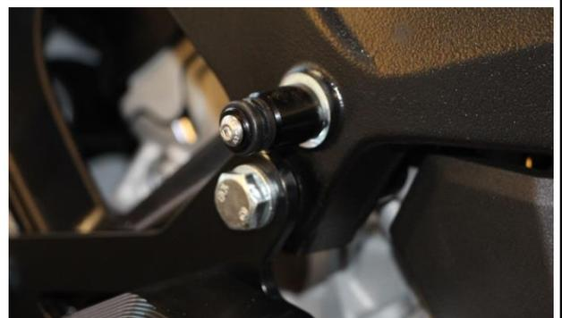
Tightening torque 4 Nm
