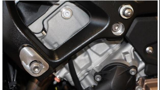
Insert the supplied spacer sleeves into the frame.
