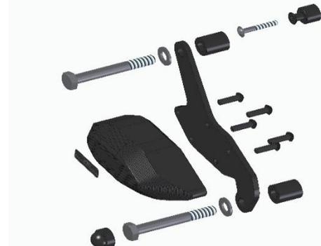
Remove the retaining screw of the fairing on the **right and left side**. Pull the rubber off the screw and press it onto the supplied spacer roller.
