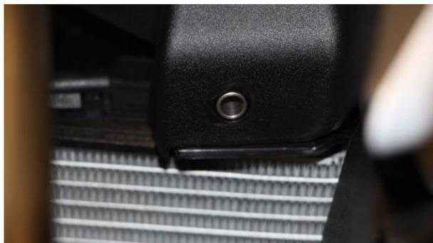
Loosen the left and right trim, pull it out of the retaining pegs and remove.
