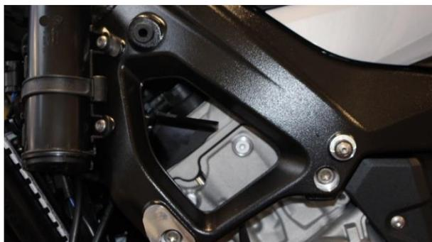
Loosen and remove both engine mounting screws on the right-hand side (these will not be reused).
