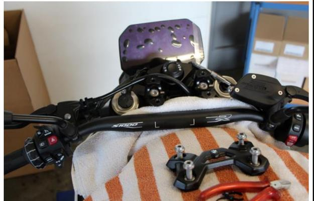
Loosen the two clamping block screws, holding the lock nuts under the fork bridge.
