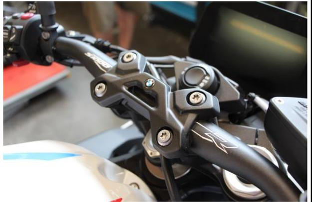
Carefully place the handlebars on the tank while pulling the clutch cable holder out of the clamps.
