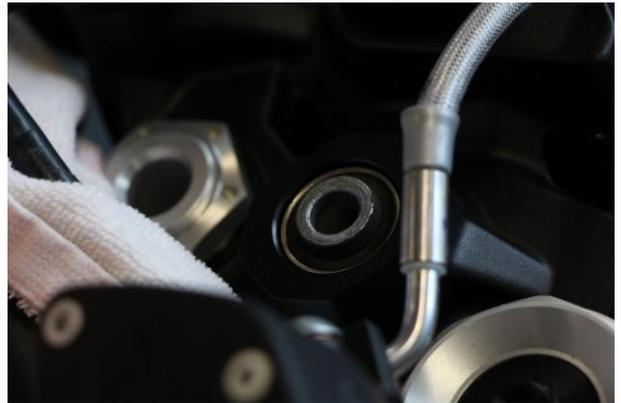
Fit the clamping brackets to the triple clamp using the enclosed raised sections and the longer screws.
