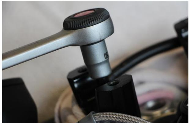
Insert the clutch cable holder and the handlebars into the clamps
